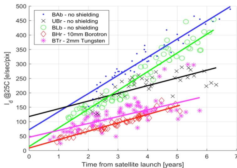
**Figure 11.** Temporal development of the CCD dark currents.
