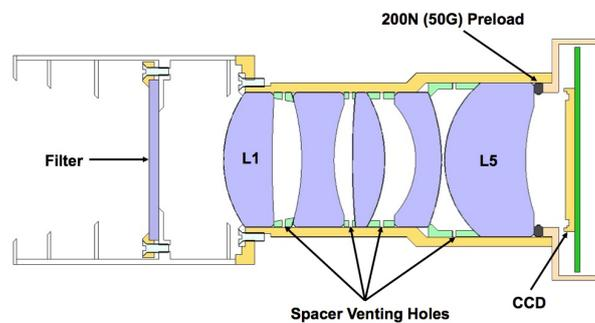
Figure 4. Camera scheme for the UNIBRITE and BRITE-TORONTO red instruments with a nearly vignetting free field-of-view of 24°. The red or blue filters are placed at the entrance pupil of the 5-lens camera to assure a constant filter function over the entire FOV. The blue cameras have slightly modified lens radii and separations to optimise the image quality for the needed wavelength range. Source: SFL
