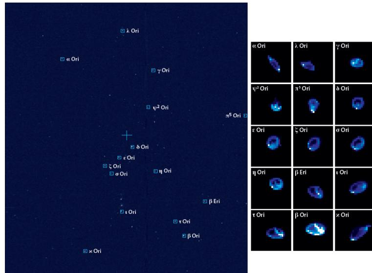
**Figure 5.** Full frame image of the Orion field taken with UniBRITE (UBr) in December 2013. The stars which have been selected for photometric time series are indicated. Subframes (24 x 24 pixels) which contain a full PSF, were stored in memory for a later download to the ground. Typical subframes in the center and close to the edge of the field are presented in the right panel.
